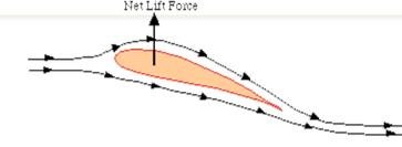
Down Force- The concept is similar to Lift Force but instead the air will have a greater flow underneath the spoiler instead of the top so this will cause the spoiler create a down force on the front and the rear of an F1 car.
