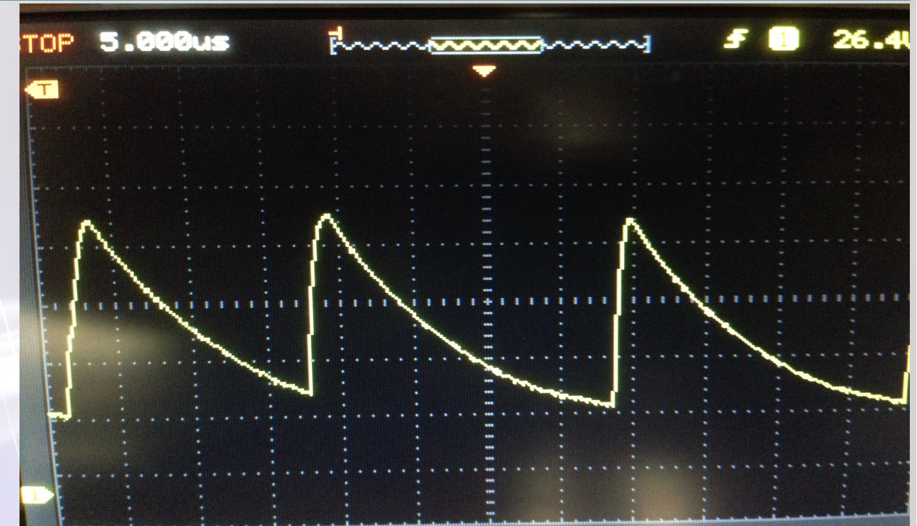
This is the display of the oscilloscope which is used to monitor photon detection events. The probes of the oscilloscope are connected across the 100kΩ resistor which is located between one end of the LED and ground. When a photon strikes the LED and current is allowed to flow through it, all of this current flows through the 100kΩ resistor to ground. This creates a measurable voltage drop across the resistor which can be interpreted as a photon detection occurrence.
