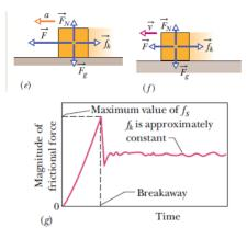
The kinetic friction force is less than the static friction force and the motion is jerky.
