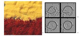
Cadmium selenide of small (top) and large (bottom) granule sizes, and a quantum corral using iron atoms.
